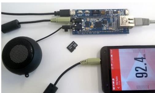
Sample Hardware Setup: The NGX board records audio data stream provided by an FM radio. A speaker is connected to the audio output for playback. An Ethernet cable connects the board to a LAN for web server access.
